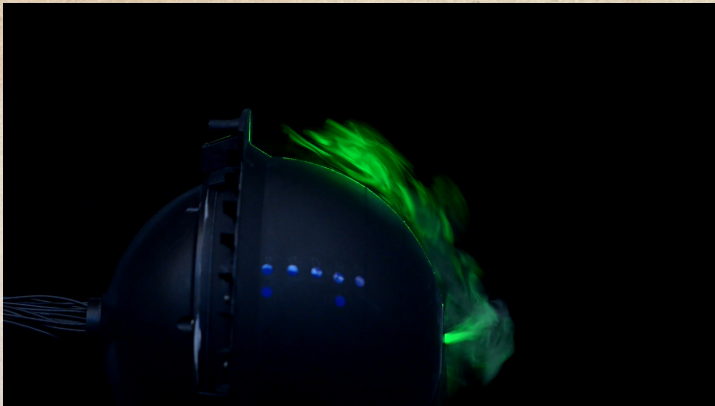
Aeroacoustic entry loads test at NASA-Ames in the Bay Area
